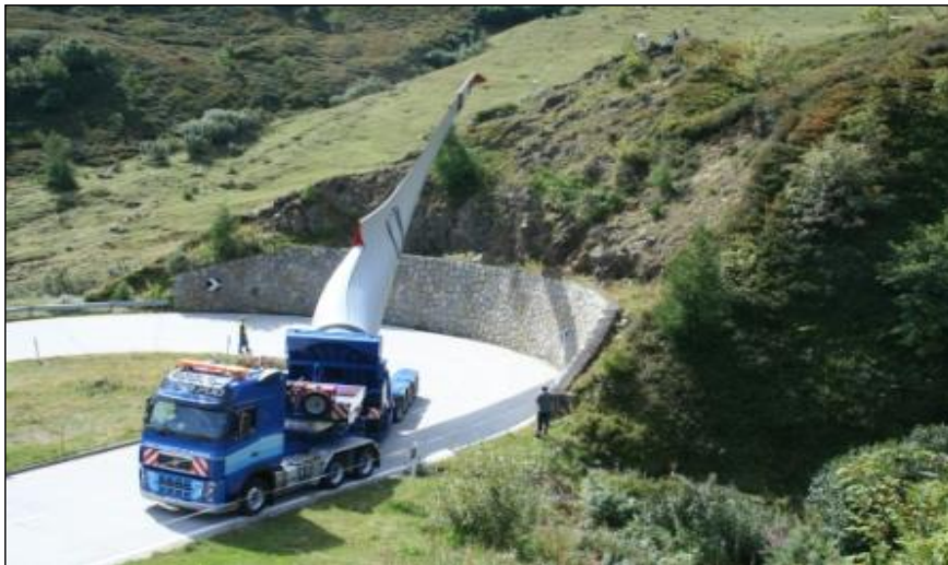
Plate 4-5 Blade adaptor transport system
